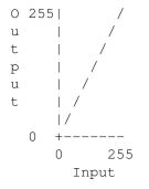
The input values are along the x axis while the output values are along the y axis. In the graph above, each input value maps onto the same output value (ie it has no effect).
