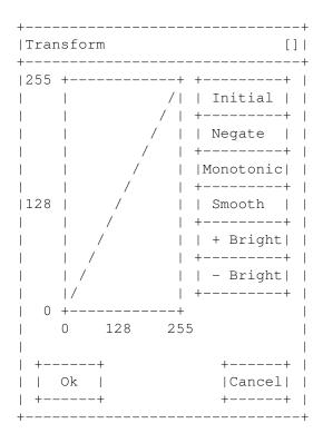
The graph shows the function that will be used, with the input values along the bottom and the out put values along the left. The shape of the function can be edited by using the left mouse button to draw straight onto the graph.
